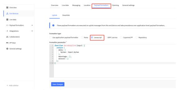
The payload decoder function for TTN V3 is here: LDDS75 TTN V3 Payload Decoder:
